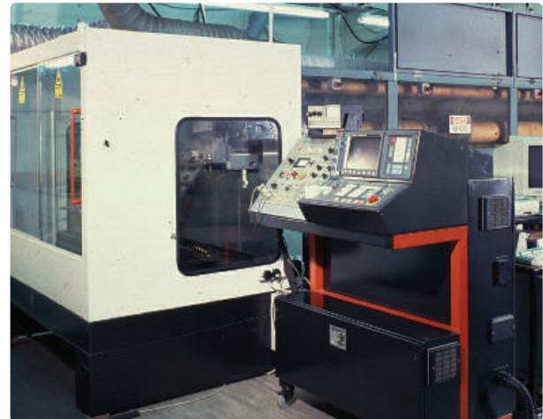
Vision panels in guarded area
