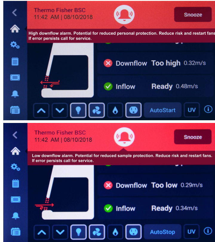
Figure 51 Alarming Screen for Downflow too high and too low Alarm
