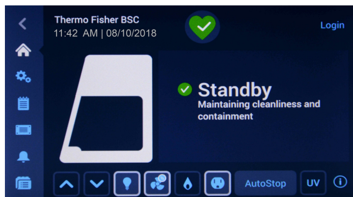
Figure 32 Main Screen - Unit in Standby
