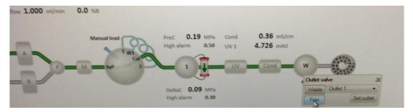
The green filled tubing in the process picture indicates the current flow of the solvent.
