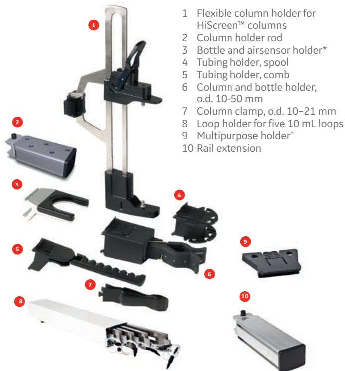
Fig 12. ÄKTA pure accessories include holders and clamps for attaching columns, flasks, and tubing to the system. o.d. = outer diameter
