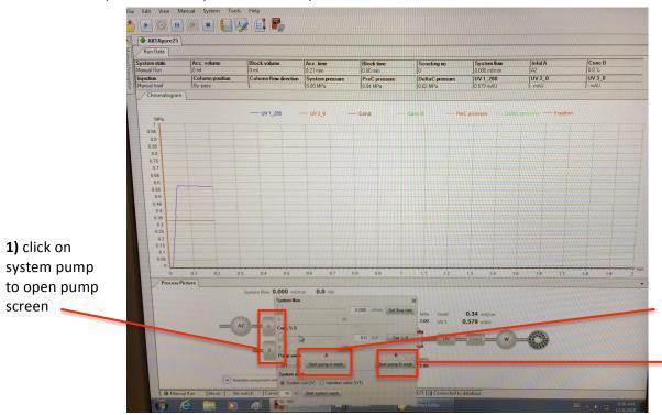
2) click pump A wash (for the selected A-inlet) or pump B wash (for B-inlet) and flush
