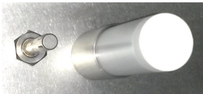
Figure 10: Plugged-in CO 2 sensor (right) and gas mixing head for CO 2
