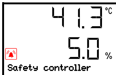
Normal display showing safety controller alarm (sample values)
