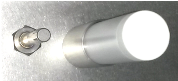
Figure 12: Plugged-in CO 2 sensor (right) and gas mixing head for CO 2
