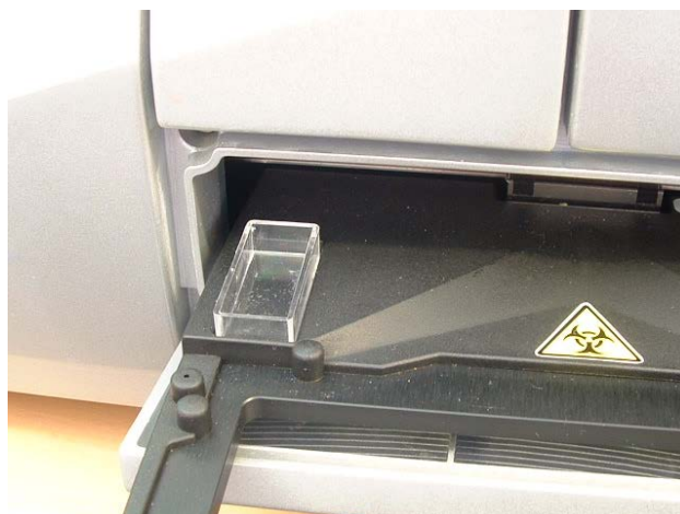
Figure 44: Waste tub on plate carrier
