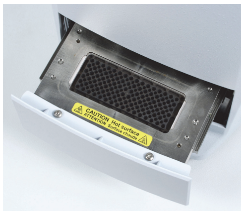
Figure 2–6. 96-well, 20 \mu l max. volume for PCR
