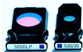
100022651 - dichroic filter holder 100022652 - bandpass filter holder
