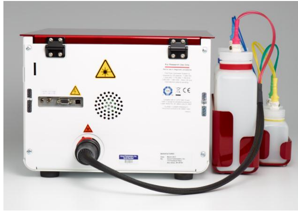
Figure 3-5. Proper Attachment of Fluidics Lines
