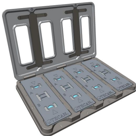
Figure 127: Cell chip adapter with springs (dark gray)
