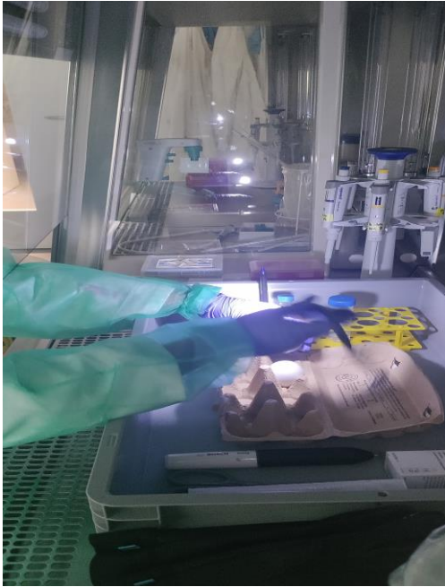
Figure 4 Tilt the egg facing the air sac, use torch to identify the spot and mark it with marker for the injection site.
