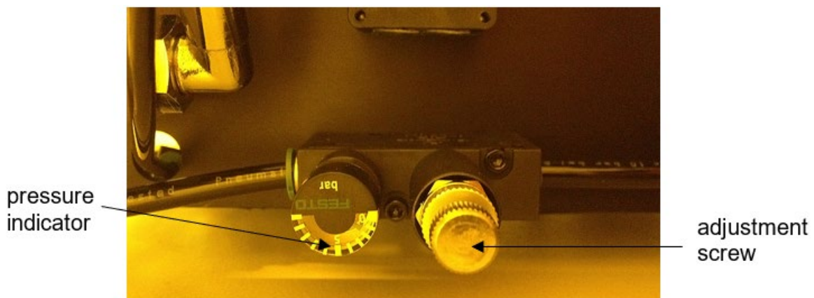
Fig. 90: Ejector pressure regulator with adjustment screw
