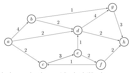
Example of a network with source "a" and sink "h" and integer capacities as indicated by the labels of the edges.
